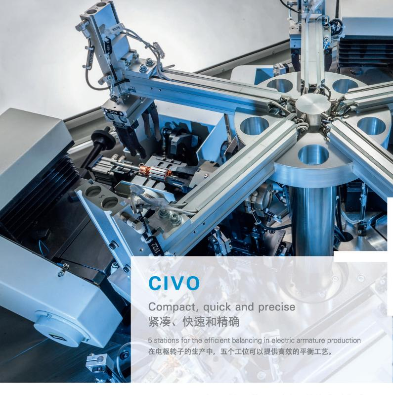
CIVO gives you maximum balancing performance in minimal space. With impressively short cycle times, electric armatures are freed from their unbalance in one process. The CIVO is designed for medium and large quantities, up to approx. 2 million electric armatures p.a.
